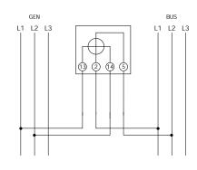
360° LED Synchroscope and Synchro Check Relay
