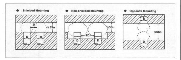
Because of possible interference of the electromagnetic fields generated by the oscillators, minimum spacing is required between adjacent or opposing "active surfaces" of proximity switches.
