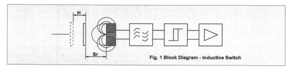
When the electrically conductive material is removed from the alternating field the oscillation amplitude increases which, by way of the electronic circuitry, will restore the switch to the original unswitched state.
