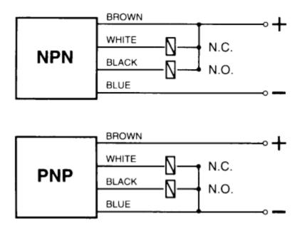
NOTE: Small rectangle Box with the diagonal line, represents the Load, Ice Cube relay Coil, PLC input channel, Input to a counter Meter.
