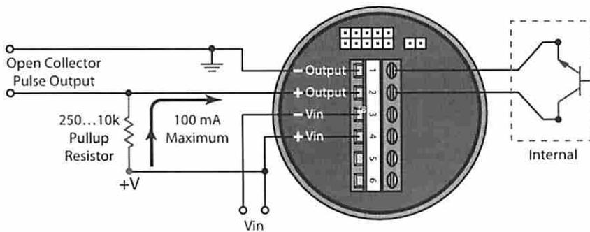
Figure 4: Wiring schematic using an external pullup resistor
