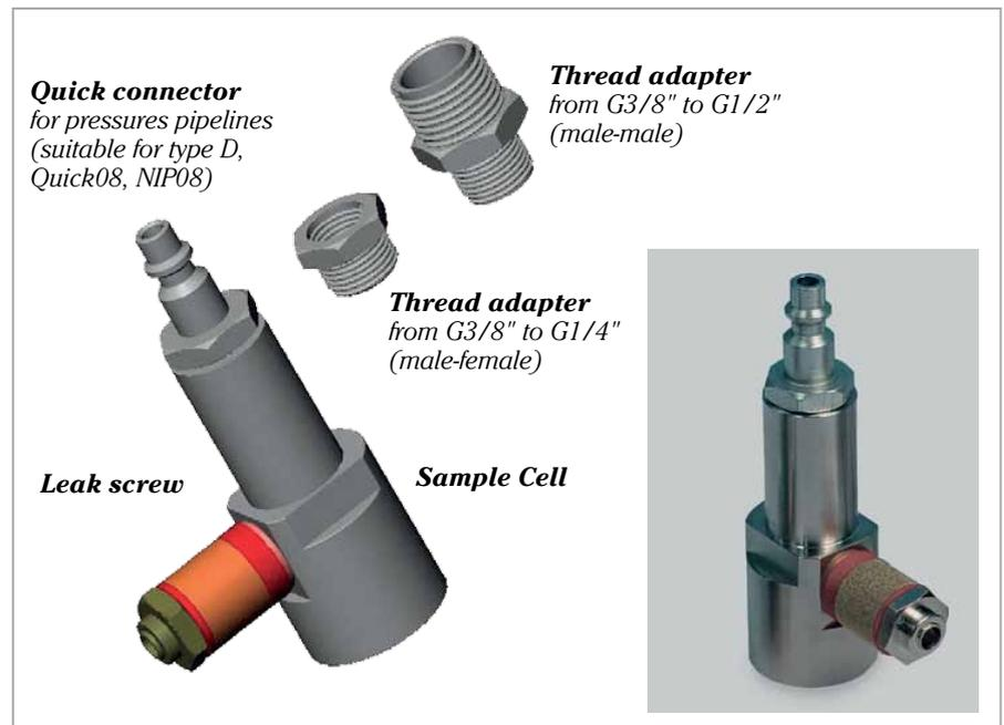
**DSC74B Sample Cell - a two-pressure model for gas pressure and atmospheric pressure furnished with inlet/outlet valve and inlet/outlet connection for gas tubing**
