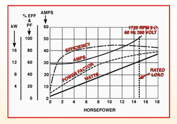
This is a chart showing the changes in performance of a 15 horsepower, 208 VAC, 1800 RPM base speed squirrel cage motor. As you can see the current changes little between no load to about four horsepower. After that, the current increases almost linearly as the load increases.
