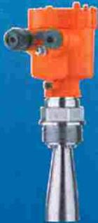
The versatile NCR-25 offers three versions for vessel heights of up to 49, 65, or 114 feet for unclassified areas or with FM and CSA hazardous location approvals. Mounting options include a 1.5", 2.0", or 3.0" NPT or a 2", 3", or 4" flange. Different seal materials address temperature requirements with a range of up to 266°C or 482°C for high temperature environments. Aluminum, plastic, and stainless-steel single and dual chamber housings are available.
