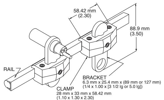
**AC227** Large, right-angle, stainless, mounting bracket (for 18 mm barrel sensors)
