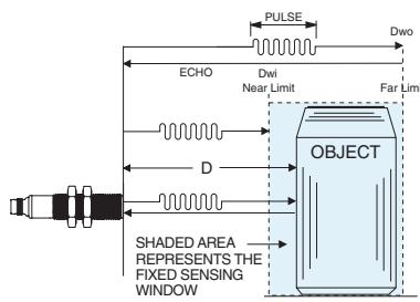
If  $D$  is within these limits, an output is generated. The output remains on until the echo does not return or it returns from outside the window limits.
