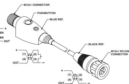
**AC132** Right-angle, M12 micro, 4-conductor, connector/cable assembly, 5 m (16') (for flat-profile connector-style sensors)
