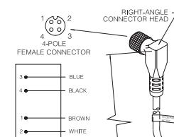
**PB100** In-line accessory push-button for teaching window limits (for Virtu series sensors).
