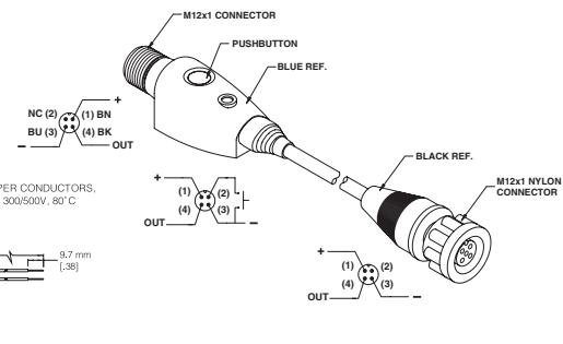
**AC132** Right-angle, M12 micro, 4-conductor, connector/cable assembly, 5 m (16') (for flat-profile connector-style sensors)
