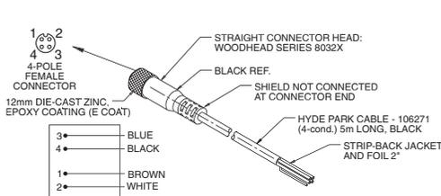
**PB100** In-line accessory push-button for teaching window limits (for Virtu™ series sensors).
