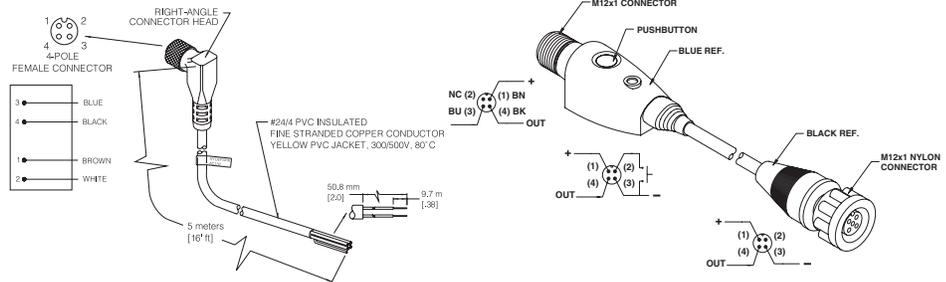
**AC132** Right-angle, M12 micro, 4-conductor, connector/cable assembly, 5 m (16')
