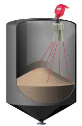
The 3DlevelScanner provides an accurate three-dimensional profile of the top surface within a storage vessel. This is beneficial when there are variations in the material surface due to multiple fill and discharge points, or with materials such as powders that do not fill/discharge symmetrically.
