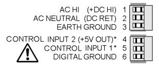
**Warning:** Hazardous voltages may be present on pins 4, 5 & 6 of P1 since digital ground is tied to pin 3 of P5 (-Signal Input). Keep pin 3 close to earth ground to minimize common mode voltage or shock hazard at pins 4, 5 & 6 of P1.
