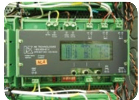
The LCD display shows the data points sent to a controller via network communication. The LEDs show proper network activity..
