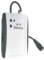
E) PN: Model AC443 Sensor Power Pack Provides 18VDC power for most sensors via M12 connector. Provided with on-off switch, LED's, and variable analog indication. Includes pushbutton for limit/span setting of VM1/18/30/80 sensors.
