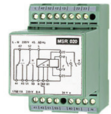
L) MSR Latching Relay, for Dry Contact Control Inputs, and Providing Relay Outputs for ON/OFF Pump Control.
