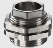
ACCTTAM25 Thread adapter M12x1 to M25x1.5 incl. 2 mounting nuts
