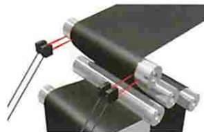
Measuring of rubber sheet thickness at calendar roller
